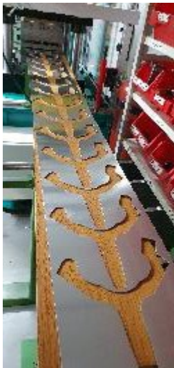
Image 2: In the first step, the Y-shaped blanks are punched from a 1.5-millimeter strong aluminum band. For the second step, the operator changes the tool in the press and is able to bend the blanks to become switching handles.
